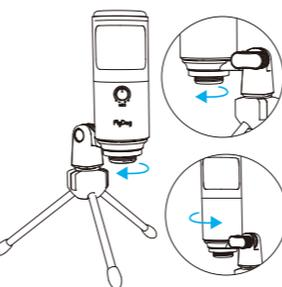
4. Screw the threaded metal ring to adjust microphone angle 360° horizontally.
