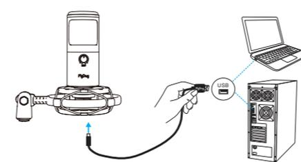
5. Connect the microphone to the computer. Plug the microphone connector into the rear back USB port of your computer.
