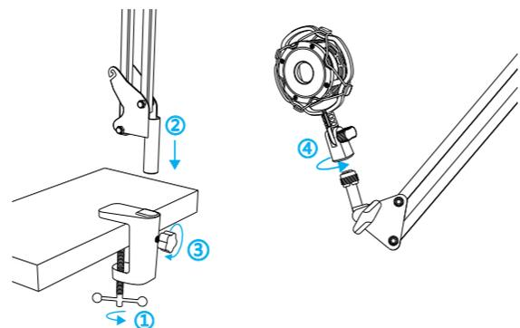
1. Screw the lower part of the C-clamp until it is tight and secure.
